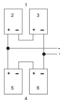
Solar panel wiring in series/parallel circuit
