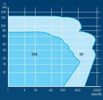
Grundfos TP/TPE is a comprehensive range of high efficiency In-line pumps. They feature the world-renowned Grundfos Blueflux® motor as standard and the TPE has an integrated frequency converter that ensures maximum efficiency at all times.
